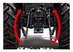
**External Hydraulic Cylinder** RX tractor has two external hydraulic cylinders which improves lift capacity with easy and convenient maintenance.
