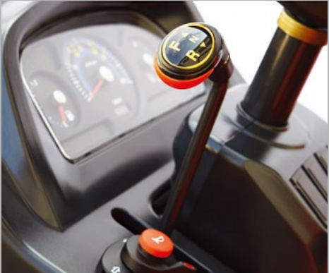
H-shuttle Applied the H-shuttle, the Daedong's unique technology • No fatigue on your left foot with no-clutch direction change • Available for H-Shuttle Model
