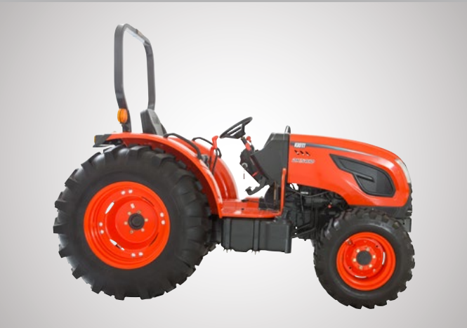
Compact Clearance It is possible to work and make turn at compact greenhouse (Width:8m, Min.height:1.2m) Outstanding engine torque makes possible to work with 190 inch rotary tiller. • Weight : 1,550Kg (Reduced the fuel consumption) • Wheelbase : 1,810mm (Improved towing capacity)
