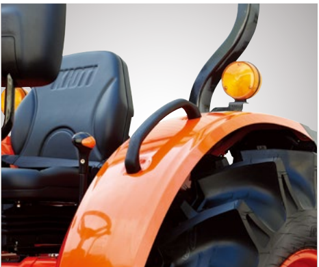
Fender Grip Armrest type handle grip on the fender will reduce the fatigue especially for the long time driver.It is possible to adjust the fender heights in accordance with the tire size.
