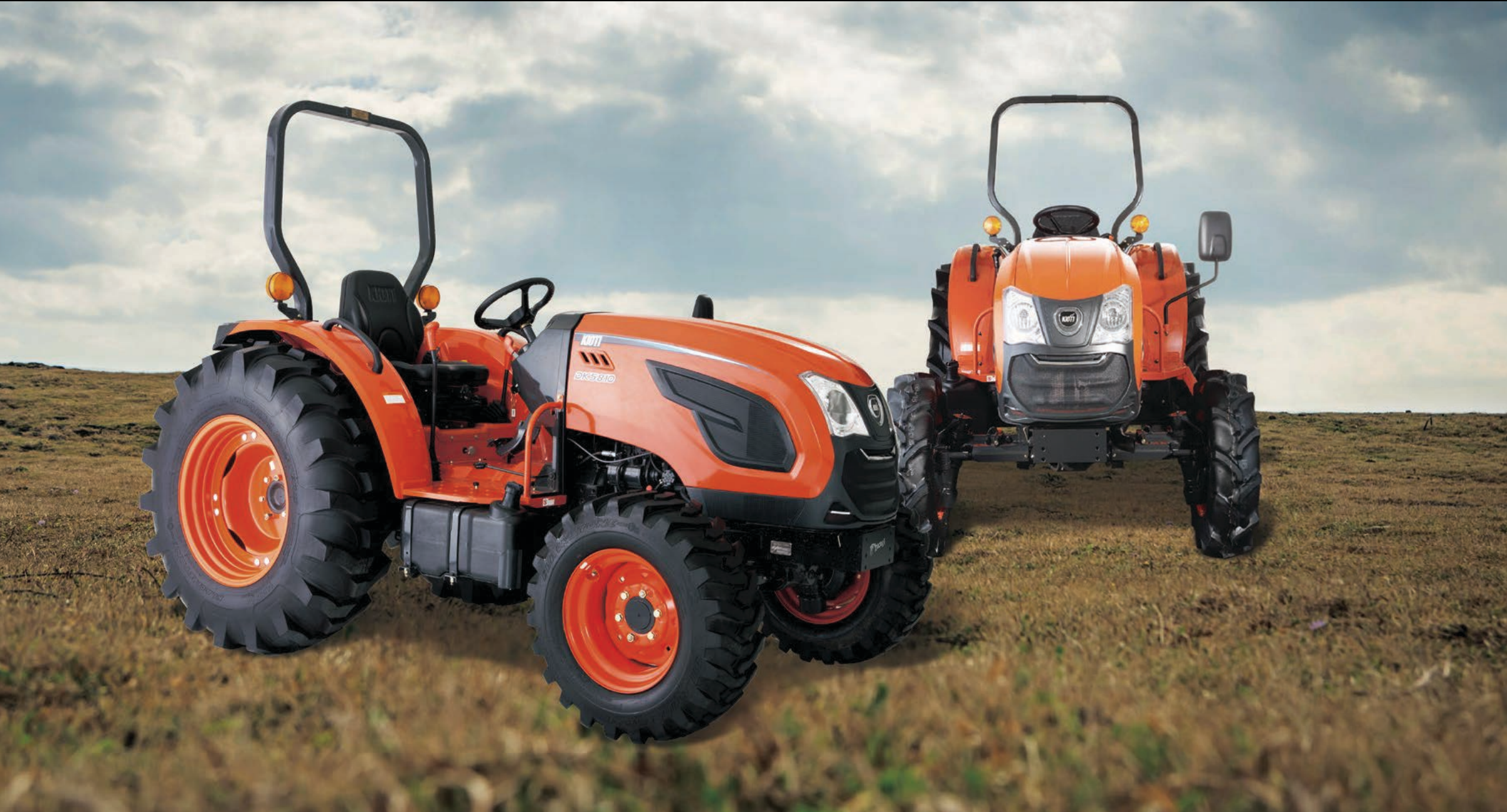
Innovative Design Center marker on the bonnet ⇒ Improve the linearity while plowing the furrow Air cylinder support system applied at the bonnet ⇒ For easy maintenance and convenience
