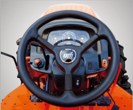
Handle The lowest height of steering wheel (1,410mm) compare to competitors ⇒ Real low profile tractor The height of steering wheel is 1,475mm The high technology digital dashboard ensures; • Better visibility even in the daytime • The CAN communication from dash to ECU Most of control buttons are located right in front of the driver for easy control
