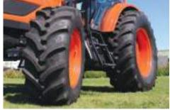
**Standard Wide Radial Tires** Standard front 440/65R24 and rear 540/65R34 tires provide high flotation and traction.
