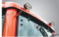
**Front and Rear Work Lights** Adjustable front and rear work light allow the operator to maneuver safely in low light conditions.
